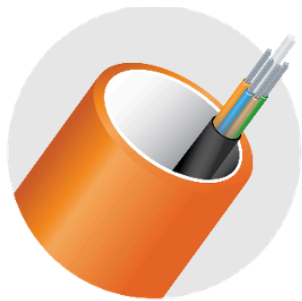
Standard Conduit with a single fiber cable
