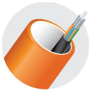
Standard Conduit with a single fiber cable
